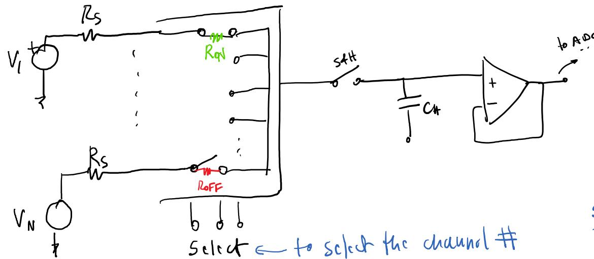
$$f_{\text{channel}} = \frac{f_{\text{sumax}}}{N} \rightarrow \text{Shannon} \quad f_{\text{in,max}} = \frac{f_{\text{channel,max}}}{2}$$
