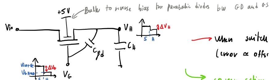
When switch open we have a charge injection due to parasitic capacitance  $C_{pd}$
