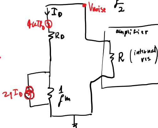
$$\frac{V_{noise}^2}{\Delta f} = \frac{2qI_0}{R_D} \left( \frac{1}{f_m} + R_D + R \right)^2 + 4kTR_D \left( \frac{R}{R + 1/f_m + R_D} \right)^2$$
