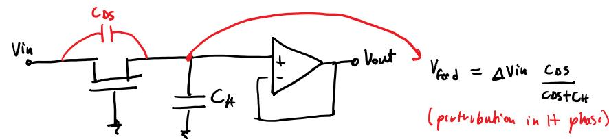
$$V_{\text{Feed}} = \Delta V_{\text{in}} \frac{C_{GS}}{C_{GS} + C_H}$$
