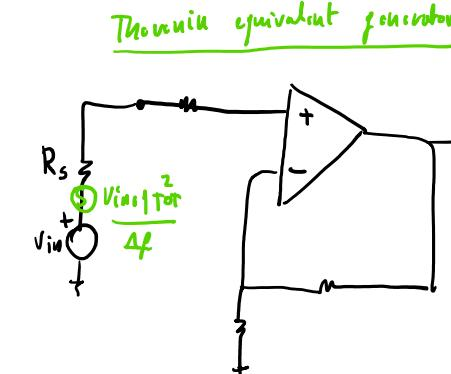
$$\frac{V_{inj,Tot}^2}{\Delta f} = 4kTR_s + \frac{V_{inj}^2}{\Delta f} + \frac{i_{inj}^2}{\Delta f} R_s^2$$
