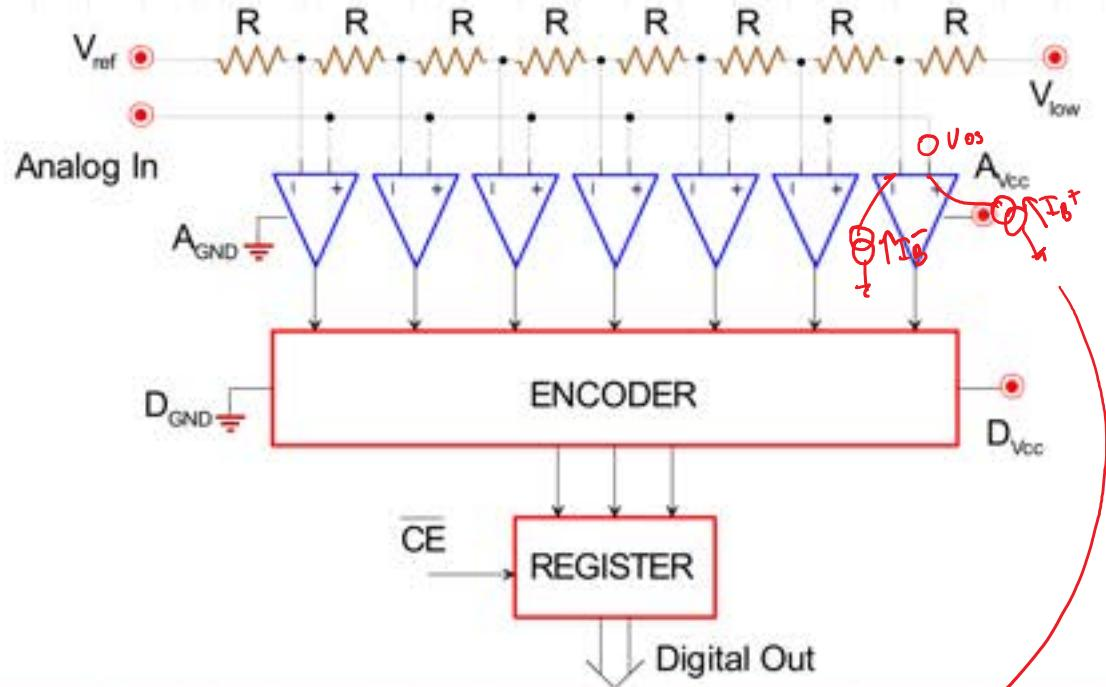
offset errors → for low value of LSB, offset can be comparable to a level and result in missing codes
