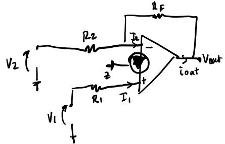
$$I_1 = \frac{V_1}{R_1} \quad I_2 = \frac{V_2}{R_2} + I_{\text{out}}$$
