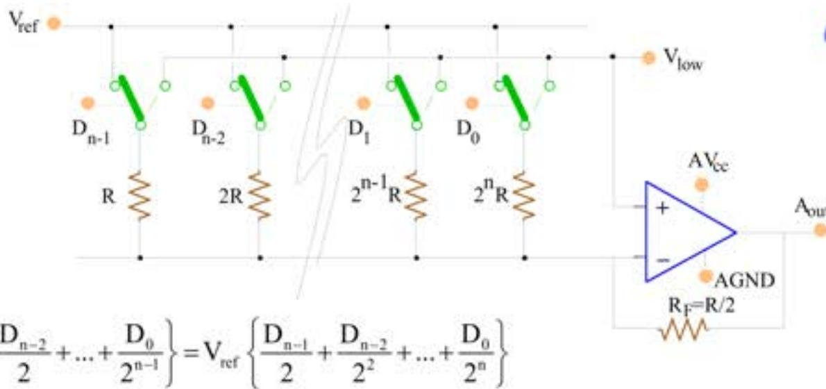
$$V_{out} = V_{ref} \frac{R_f}{R} \left\{ \frac{D_{n-1}}{1} + \frac{D_{n-2}}{2} + \dots + \frac{D_0}{2^{n-1}} \right\} = V_{ref} \left\{ \frac{D_{n-1}}{2} + \frac{D_{n-2}}{2^2} + \dots + \frac{D_0}{2^n} \right\}$$
