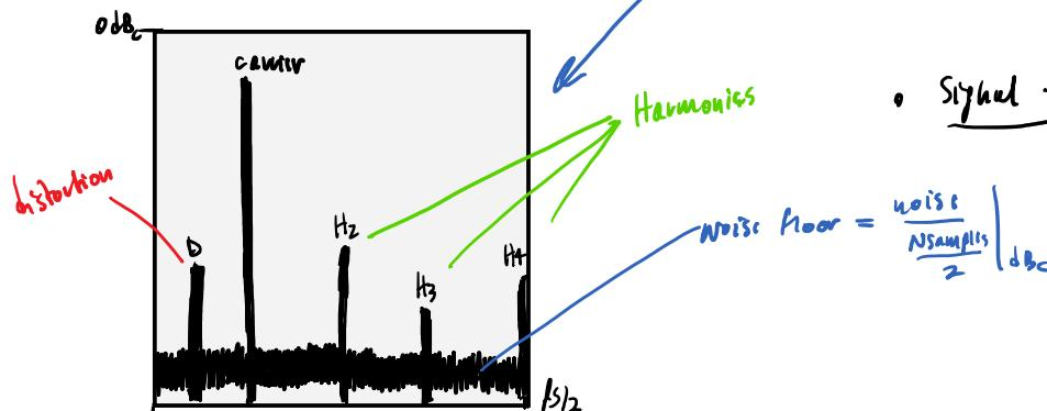
Total Harmonic Distortion:  $THD = \frac{\text{power of all the harmonics}}{\text{power of useful signal}} | dB$
