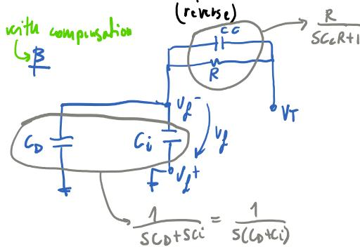
$$V_f^- = -V_f = \frac{1}{s(C_D + C_i)} V_T = \frac{1}{s(C_D + C_i) + \frac{R}{sC_C R + 1}} V_T = \frac{sC_C R + 1}{s(C_D + C_i)R + sC_C R + 1} V_T$$
