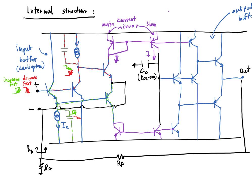
$$f_{pole} = \frac{A_{out}}{2\pi \left[ R_F + \left( 1 + \frac{R_F}{R_B} \right) R_B \right] C_C}$$
