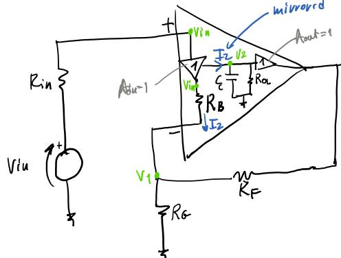
$$I_2 = \frac{V_{in} - V_1}{R_B} = \frac{V_1}{R_B} + \frac{V_1 - V_{out}}{R_F}$$
