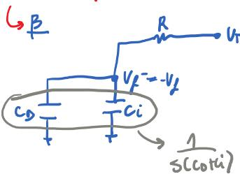
$$V_f^- = -V_f = \frac{1}{s(C_D + C_i)} V_T = \frac{1}{s(C_D + C_i) + \frac{R}{sC_C R + 1}} V_T$$
