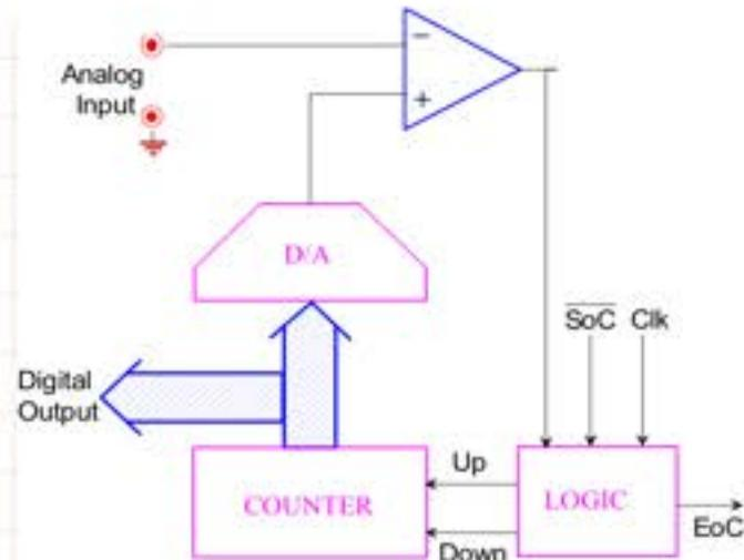
Components: 1 DAC, 1 counter, 1 comparator, 1 up/down logic
