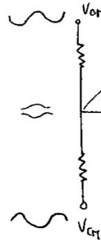
If the capacitance of the cables is not equal, the transfer function of  $V_{CM}$  is different. Let's suppose the CM is the same; if the time constants  $R \cdot C$  are different, the signal which is supposed to be cancelled it is not cancelled at all, because the same signal is modified on the two branches. So even a mismatch in the shielding of the two cables may result in a catastrophic effect because on common mode we provide two different signal paths.
