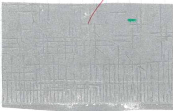
extreme case of damaged silicon
