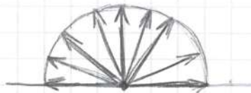
uniform (isotropic) emission from a point source
